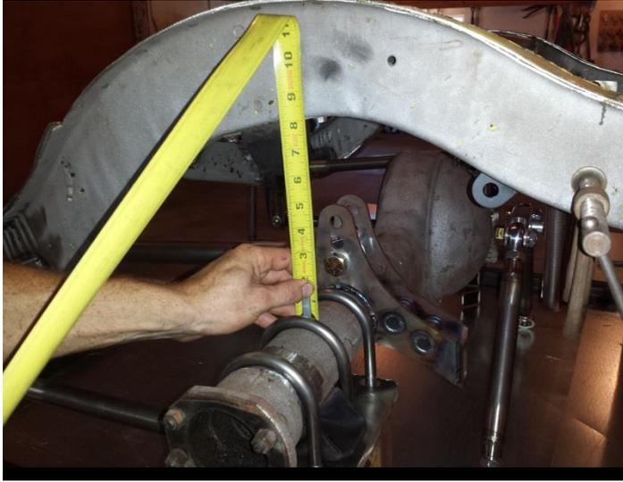
measure both sides to make sure they're the same, lower bars should be level, or very close, if not, make adjustments at this time to them by moving up or down in the link holes on the front bracket. Once that's done, set the pinion angle to 1 degree negative. (Pinion pointed down is negative)
