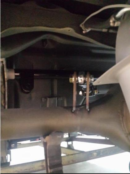
Next, tack the tabs in place, make sure to put some good heavy tacks on. Now, recheck all measurements, once this is done, and everything looks good, you can weld the tabs on, weld all the way around for maximum strength, once again, be careful, and take your time welding as to not get the housing too hot, getting the housing too hot from welding can distort the axle tubes.
