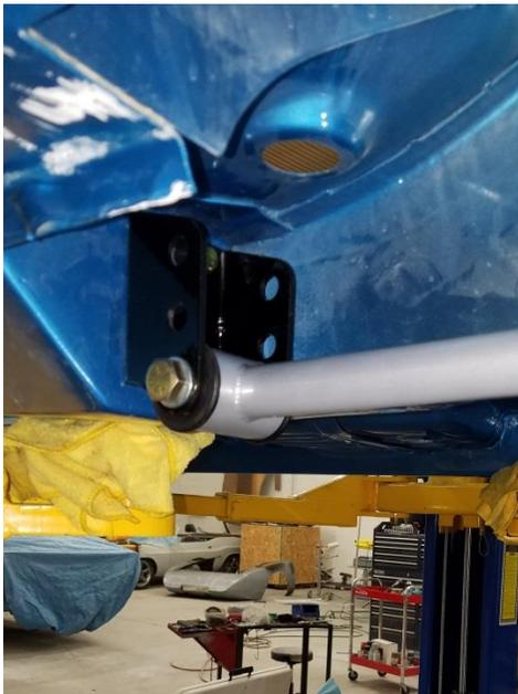
Now That everything is bolted up as you see in the picture above,bolt the lower forward link brackets into the factory spring mounting location using the 4 bolts provided,per each side.
