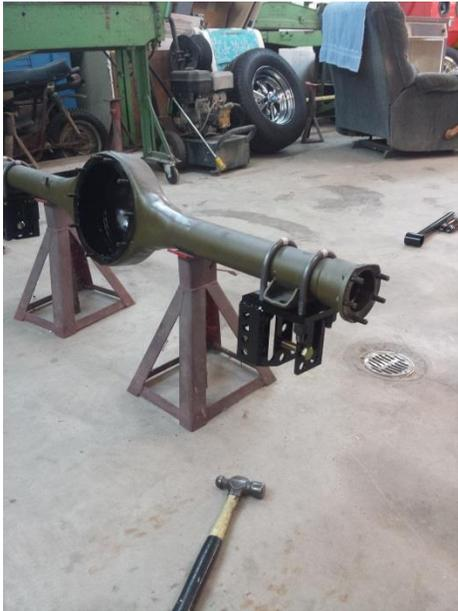
Next, bolt the lower brackets onto the housing using the supplied u-bolts,snug down hand tight for now.
